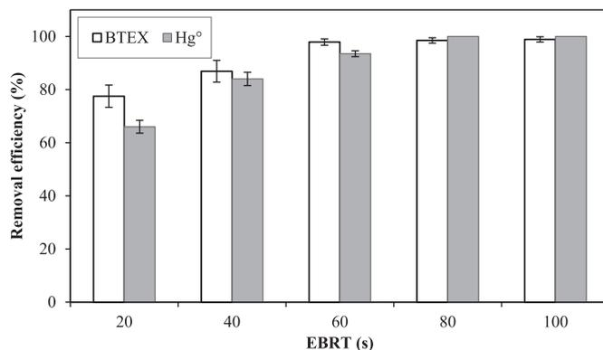
Fig. 2. Average BTEX and Hg° removal efficiency of the biofilter at different EBRTs (n = 15, BTEX = 3.25 g/m<sup>3</sup>, Hg° = 0.35 g/m<sup>3</sup>).
